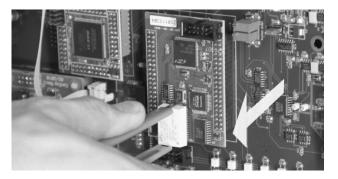
4. Put on the new battery. Ensure correct orientation (locking pins).
