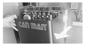
2. Switch machine power ON (LED on Pacemaker<sup>™</sup> board green) ATTENTION - DON'T TOUCH OTHER PARTS!
