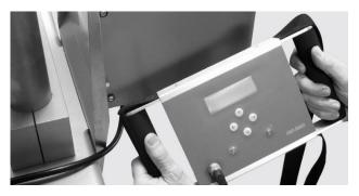
6. Switch machine power OFF Discharging - wait at least 5 min. before proceed with step 8.
