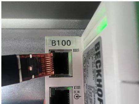
3. Connect the additional network cable between control IPC and host PC (Laptop).
